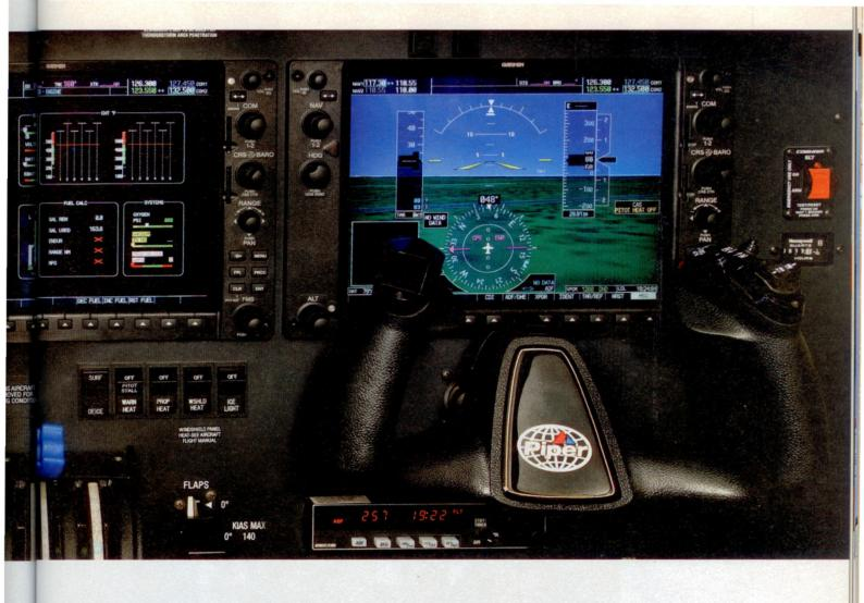
A GARMIN G1000 integrated cockpit (above) and Aspen Avionics standby system (above far left) supplant the Seneca's previous dual G600 panel (left). A comfortable cabin includes leather seats, cup holders, a cooler integrated into the arm rest, and convenient intercom jacks.
