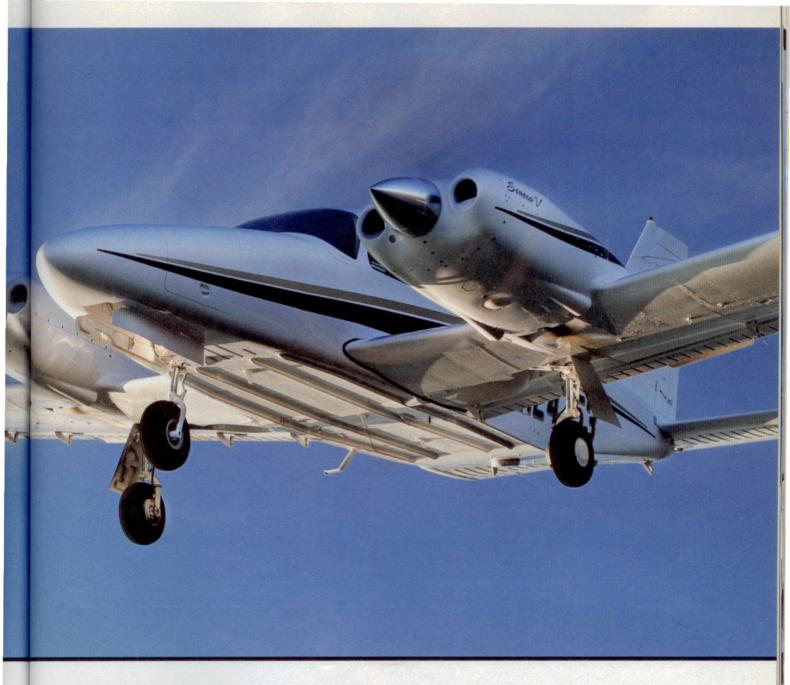
LOADS OF DOORS and more give the Seneca V lots of stowage. A big door allows access to nose baggage (top left). Dual doors provide convenient access to the cabin and aft baggage. A door atop the left nacelle opens when the air conditioning system is engaged. Typical Piper, the simple hydraulic landing gear free-falls if pressure is lost (above); no need to crank the gear down.
